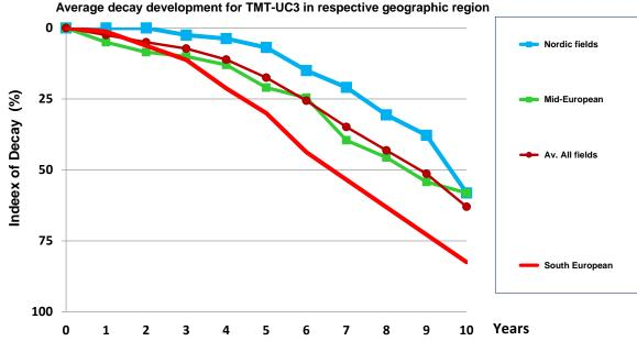
Figure 3: Performance of UC3 grade thermally modified spruce (TMT-UC3) in different regions of Europe.
