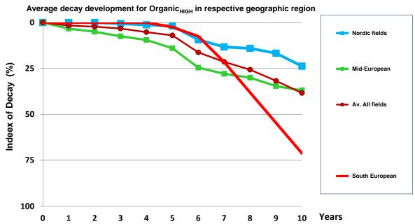
Figure 4: Performance of stakes impregnated with organic preservative to high retention level (levels intended to simulate levels for UC4 that had been obtained from EN 113 tests) in different regions of Europe.
