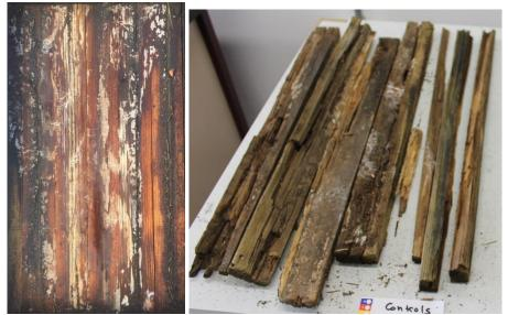
Figure 5: Decay in TMT-UC2 stakes in deck in UK and what remains of Control stakes in Italy after 10 years.
