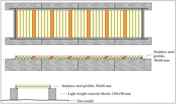
Figure 1: Test rig for double layer test.
