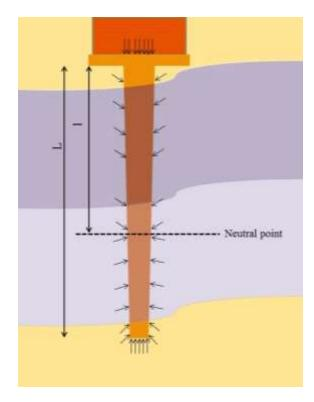
Figure 7. Location of the neutral point in a timber pile in service (sand layers are yellow, weak layers purple, orientation of the load on the pile is given by arrows)
