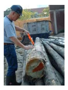
Figure 4. Extracted piles to be inspected and measured over their full length
