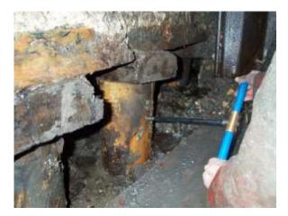
Figure 6. Increment borer (diameter 10 mm)
