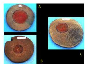
Figure 3. Example of variation in wood structure in pine pile heads of app. 16 cm in diameter. A and B show differences in sapwood width and C shows a asymmetric pith and compression wood at the right side
