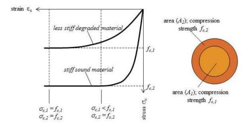
Figure 8. Effect of ductile behaviour (wood loaded in compression)
