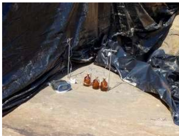
Figure 4 Impression of the sampling and measuring equipment when installed. The embankment and the ship are now completely covered in black plastic to protect them from damage by drying out.
