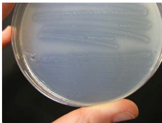
Fig. 9. Cellulolytic bacteria cause clearing zones on cellulose agar. These bacteria are not able to degrade wood, but are present in the microbial community surrounding erosion bacteria.
