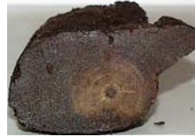
24: Foundation Bryggen, Sweden. Sample 2 Pine
