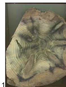
1: Foundation Amsterdam, the Netherlands; Sample 1d, Pile 3, ;Height 0;Spruce
