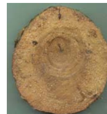
7: Pile extraction Haarlem, the Netherlands Pile 5, Height 200Poplar
