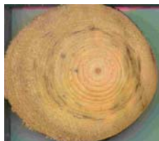
4: Foundation The Netherlands Pile 6, Height 3000-3500 Pine
