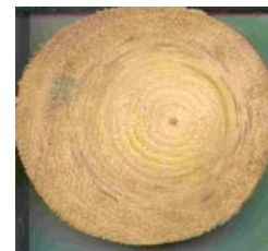
4: Foundation The Netherlands Pile 6, Height 2000-2500 Pine
