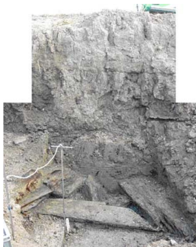
Figure 3: Soil profile in excavation pit of site 27 (lot GZ80), with the ship's wood lying at the bottom. The brown to blue-grey colour transition at the bottom of the profile represents the redox-boundary. The wood below this boundary seems to be in reasonably good condition, whereas the wood above it (to the left in the picture) is brown, crumbly and soft (instead of black and firm).
