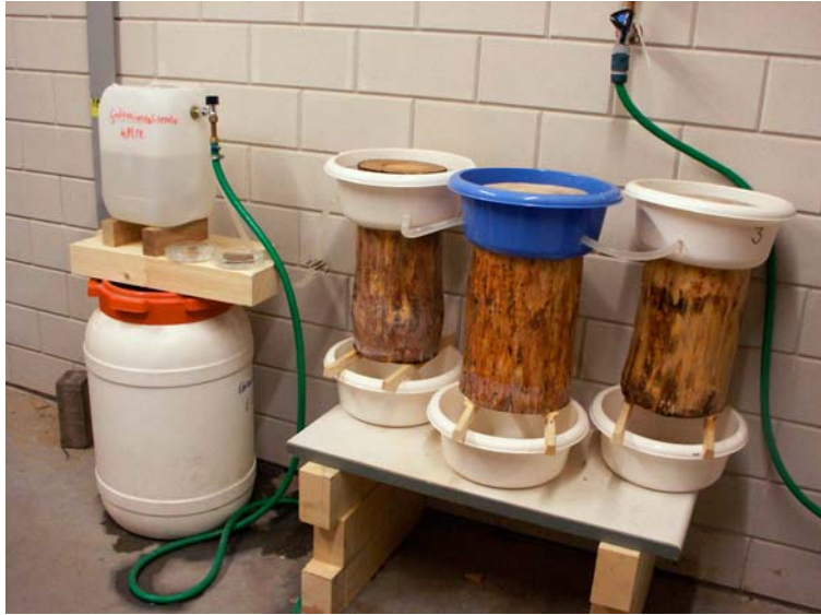
Figure 2. Test set-up experiment water flow trough bark.
