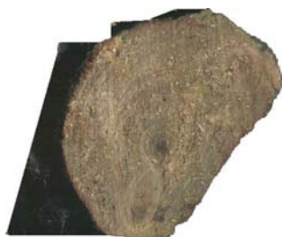
7: Pile extraction Haarlem, the Netherlands Pile 4, Height 3370 Poplar
