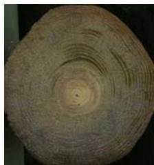
4: Foundation The Netherlands Pile 3, Height 450-920 Pine
