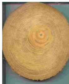
4: Foundation 4 The Netherlands Pile 5, Height 1000-1500; Pine
