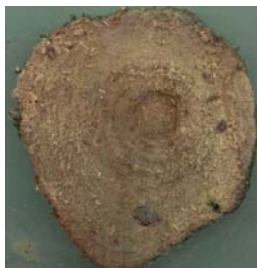
7: Pile extraction Haarlem, the Netherlands Pile 5, Height 1330 Poplar
