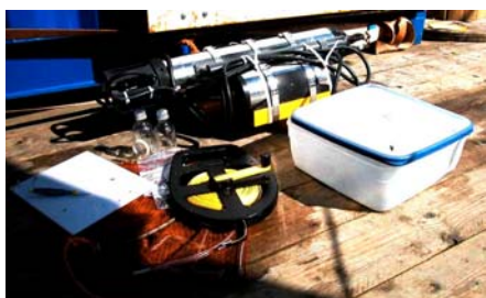
Overview of the equipment used to sample the wreck site: the datalogger, measuring equipment, 100 ml bottles for the water and sediment samples and boxes to transport the samples to the surface
