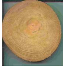
4: Foundation The Netherlands Pile 5, Height 2000-2500 Pine
