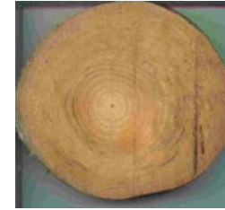
4: Foundation The Netherlands Pile 6, Height 500-1000 Pine
