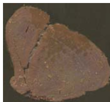
24: Foundation Bryggen, Sweden. Sample 4a-c Pine
