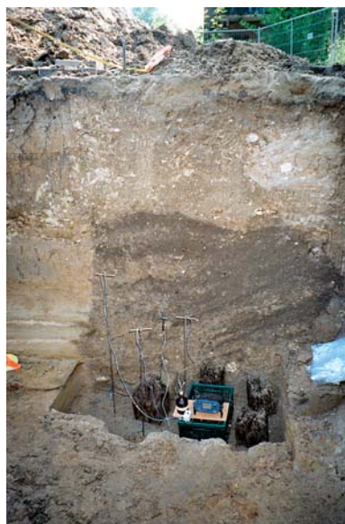
Fig. 4 Water extraction equipment and redox probe installed around the foundation piles. In the profile, the dark area is the pit that was dug top install the oil tank, which lies to the right of the piles (underneath the plastic bags).
