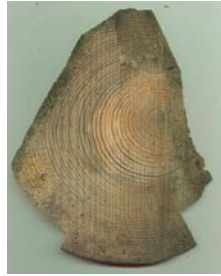
1: Foundation Amsterdam, the Netherlands; Sample 1b, Pile 3, Height 0-250Pine
