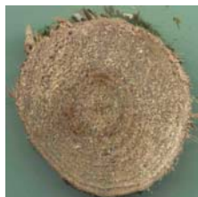
7: Pile extraction Haarlem, the Netherlands Pile 6, Height 1480 Poplar
