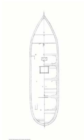
Fig 2. A reconstruction of the ship construction at the orlop-deck-level (Bohusläns museum 2003).
