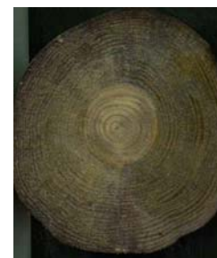
4: Foundation The Netherlands Pile 3, Height 0-450 Pine
