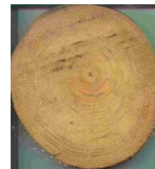
4: Foundation 4The Netherlands Pile 5, Height 1500-2000 Pine
