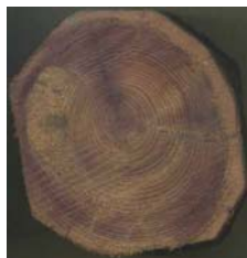
18: Foundation Venice, Italy Pile 4 Larch
