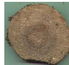
7: Pile extraction Haarlem, the Netherlands Pile 6, Height 1480, sample 2 Poplar
