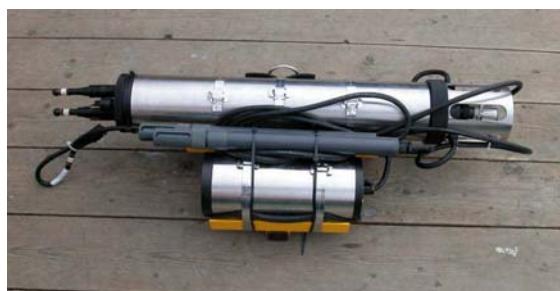
With the WaterWatch 2681 datalogger from EauxSys Ltd. data about the water and sediment conditions have been measured.
