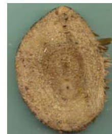
7: Pile extraction Haarlem, the Netherlands Pile 6, Height 430 Poplar
