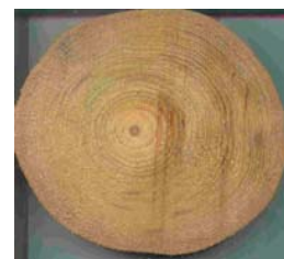
4: Foundation 4 The Netherlands Pile 7, Height 3000-3500 Pine
