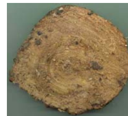
7: Pile extraction Haarlem, the Netherlands Pile 4, Height 300 Poplar
