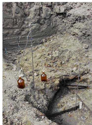
Figure 5: lysimeters and redox-probe installed in less-than-ideal locations. Lysimeter 3 and redox-probe are in the background
