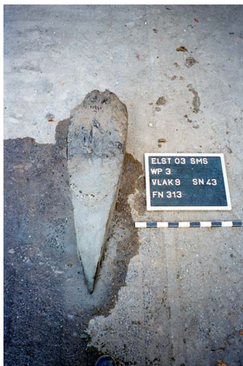
Figure 5. Largest pile (S43) taken as sample for BACPOLES. Still sticking to the pile is gravel from the coarse sediment in which it had been standing.
