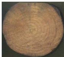
19: Foundation Venice, Italy Pile 4 Pine
