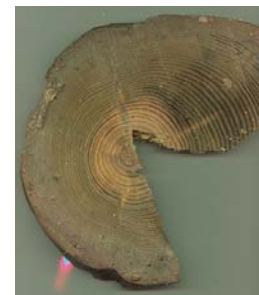
1: Foundation Amsterdam, the Netherlands; Sample 1a, Height 300-350; Pine
