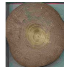
4: Foundation The Netherlands Pile 4, Height 690-1390 Pine
