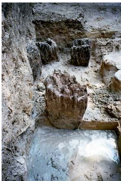
Figure 3 close-up of the largest pile sampled for BACPOLES (number SN 43; BACPOLES number 26.te.1). Soil samples were taken from the pit in the foreground, which clearly shows the ambient groundwater level relative to the piles.
