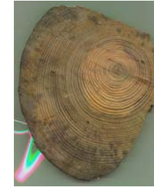
1: Foundation Amsterdam, the Netherlands; Sample 1b, Pile 3, Height 300-350; Pine
