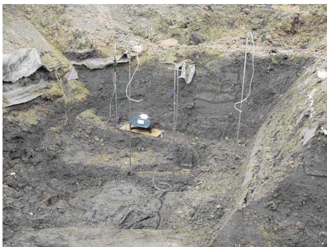
Figure 4: position of redox-probe and lysimeters (during setting-up).
