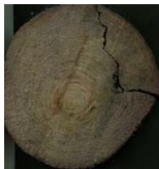
4: Foundation The Netherlands Pile 4, Height 0-670 Pine
