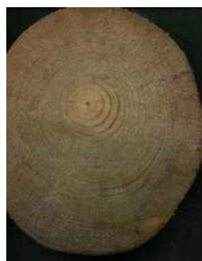
4: Foundation The Netherlands Pile 2, Height 690-1370 Pine
