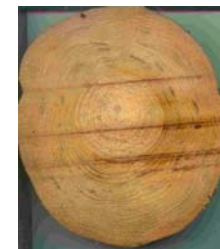
4: Foundation The Netherlands Pile 7, Height 1000-1500 Pine
