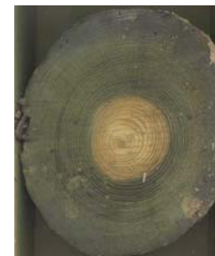
23: Foundation Leeuwarden, the Netherlands. Pile 1, Height 420 Pine
