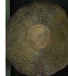
4: Foundation The Netherlands Pile 2, Height 0-690 Pine
