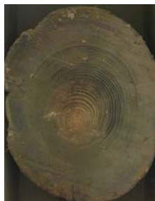
23: Foundation, Leeuwarden, the Netherlands. Pile 1, Height 120 Pine
