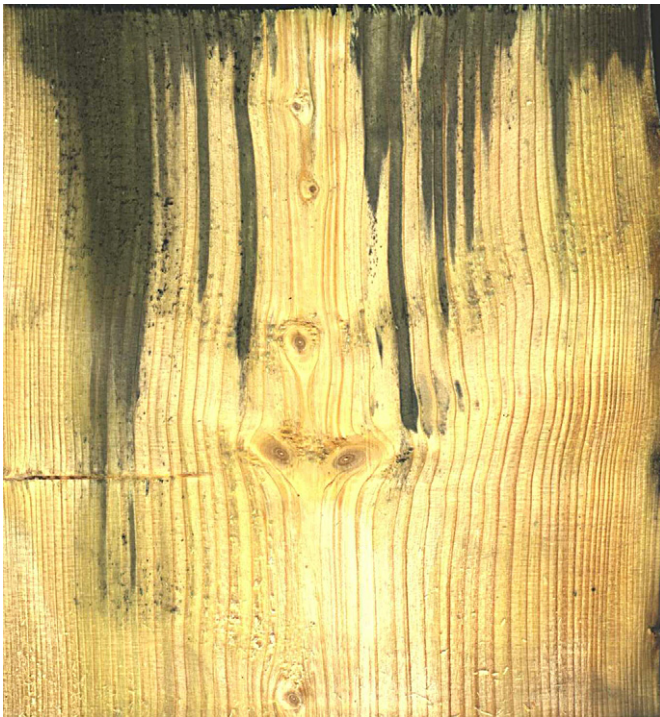
Fig. 7. Examples showing the stained water pathway in spruce.
