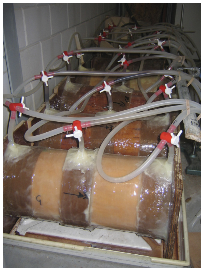
Fig. 2. Experimental design to study water flow through 450-mm-long stems under different pressures.
