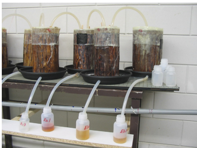
Fig. 1. Experimental design to study water flow through 300-mm-long stems without pressure.
