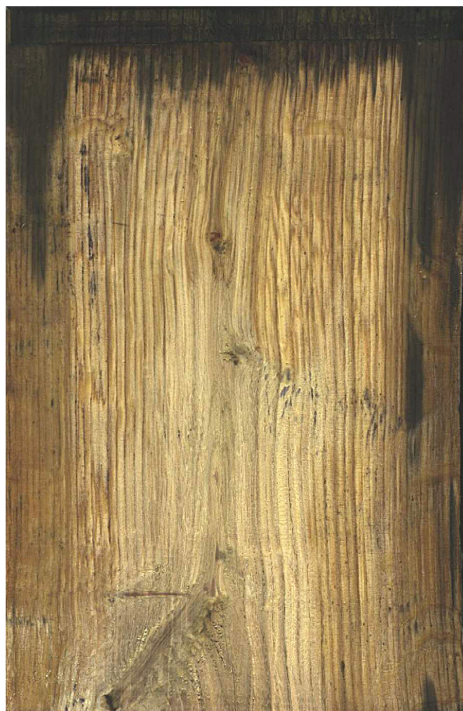
Fig. 4. Examples showing the stained water pathway in oak.
