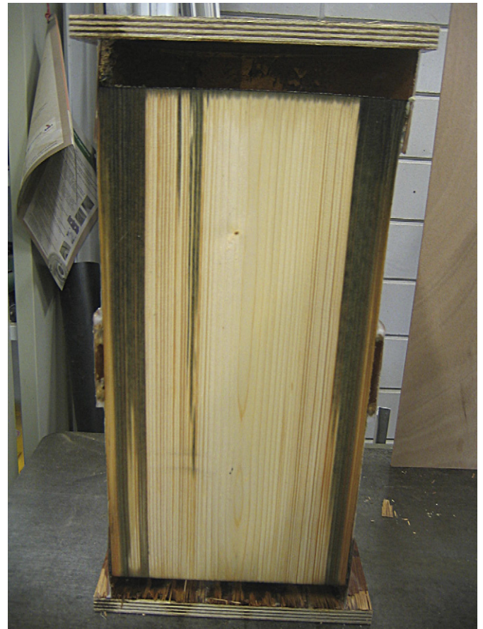
Fig. 12. Stained axial water pathway in spruce.
