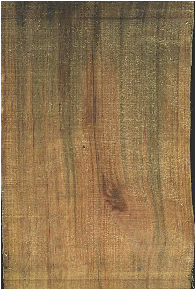
Fig. 5. Examples showing the stained water pathway in alder.
