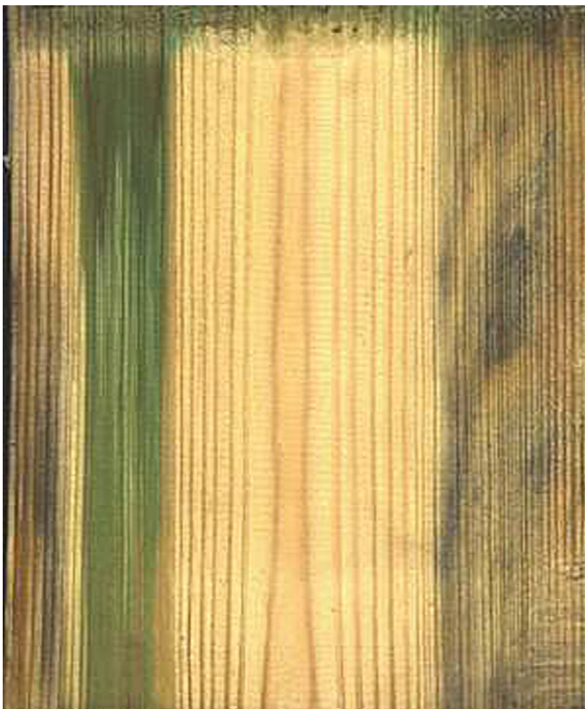
Fig. 8. Examples showing the stained water pathway in pine.
