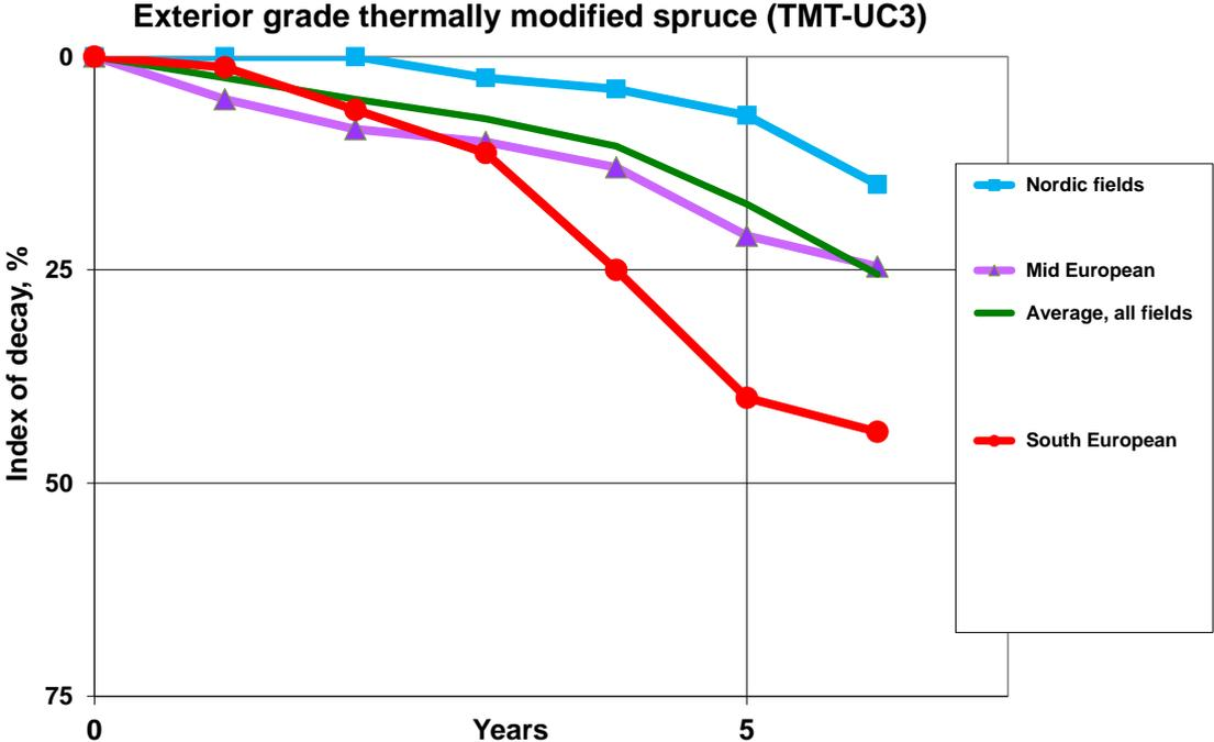
Figure 3. Performance of UC3 grade thermally modified spruce (TMT-UC3) in different regions of Europe.
