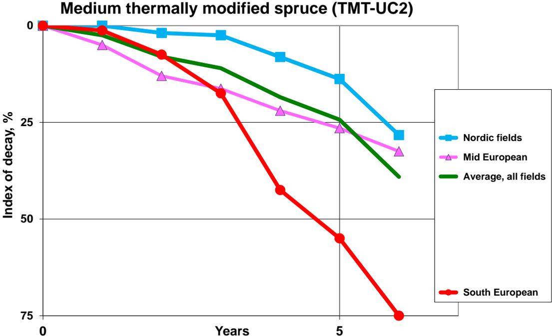
Figure 2. Performance of medium thermally modified spruce (TMT-UC2) in different regions of Europe.
