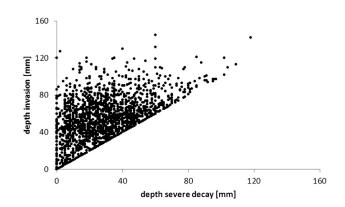
**Fig. 17.** Relation between thickness of depth of bacterial severe decay and invasion in pine (N = 1859).
