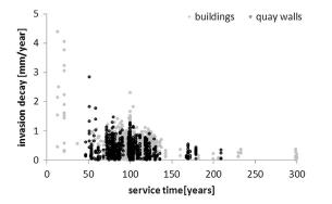
Fig. 8. Velocity of bacterial invasion in piles under buildings and quay walls in relation to service age.
