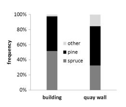
In Figs. 1 and 2 general aspects of the foundation construction under buildings and quay walls are compared. The number of piles
