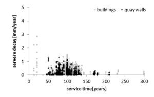
Fig. 9. Velocity of severe bacterial decay in piles under buildings and quay walls in relation to service age.
