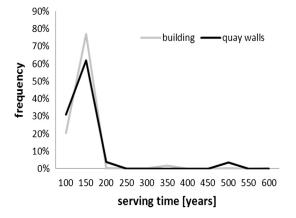
**Fig. 1.** Frequency diagram of the service time (0–100, 100–150, 150–200, 200–250, 250–300, 300–350, 350–400, 400–450, 450–500, 500–550, 550–600 years).
