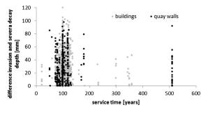
Fig. 12. Activity of decay in pine piles under building and quay walls in relation to service age.
