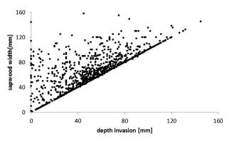
Fig. 14. Relation between pine sapwood width and depth of bacterial invasion (N = 1859).
