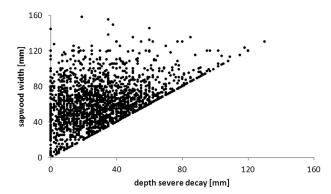
**Fig. 15.** Relation between pine sapwood width and depth of severe bacterial decay (N = 1859).
