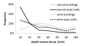
Fig. 11. Frequency diagram of the depth of severe decay in spruce and pine piles under buildings or quay walls.
