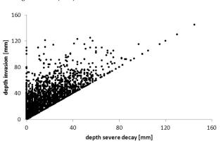
**Fig. 16.** Relation between thickness of depth of bacterial severe decay and invasion in spruce (N = 1880).
