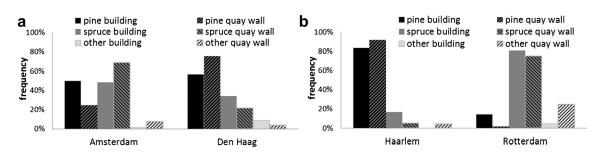
Fig. 4. Frequency diagram of the occurrence of timber species of piles under buildings or quay walls in and soil in Amsterdam, Den Haag, Haarlem and Rotterdam.
