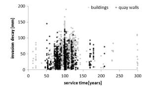
Fig. 6. Depth of bacterial invasion in piles under buildings and quay walls in relation to service age.
