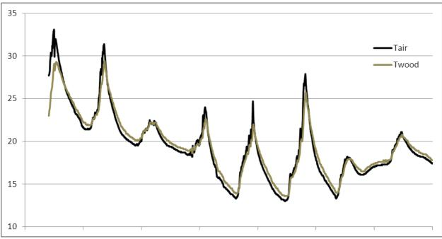
Figure 2. Variation in temperature of air and inside wood during 8-day test
