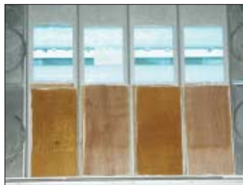
Accelerated weathering, UV with waterspray
