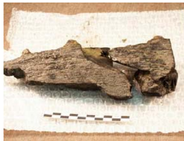
Figure 2. Fragment of wood with iron nails; iron sulfides - a lustrous gold color - have formed in a crack inside the wood.
