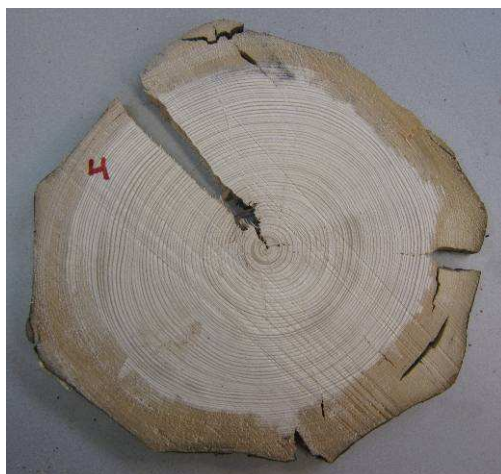
Figure 8: disk (Ø 160 mm, ca. 70 yearsrings) from one of the piles underneath the Royal Palace on the Amsterdam Dam square which was 350 year in service
