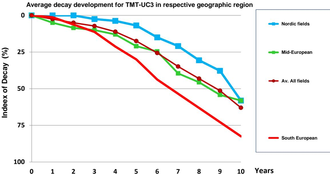
Figure 3: Performance of UC3 grade thermally modified spruce (TMT-UC3) in different regions of Europe.
