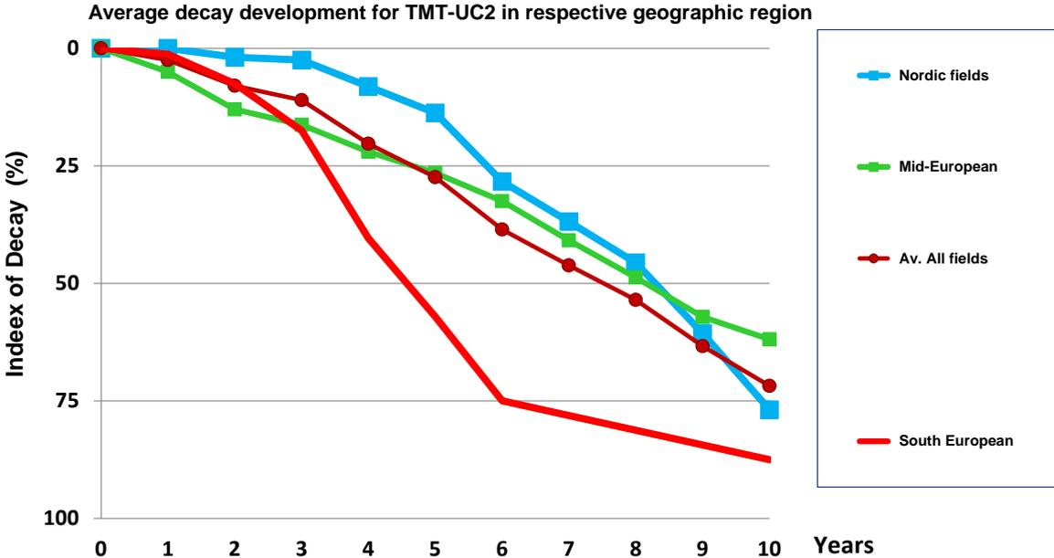
Figure 2: Performance of medium thermally modified spruce (TMT-UC2) in different regions of Europe.
