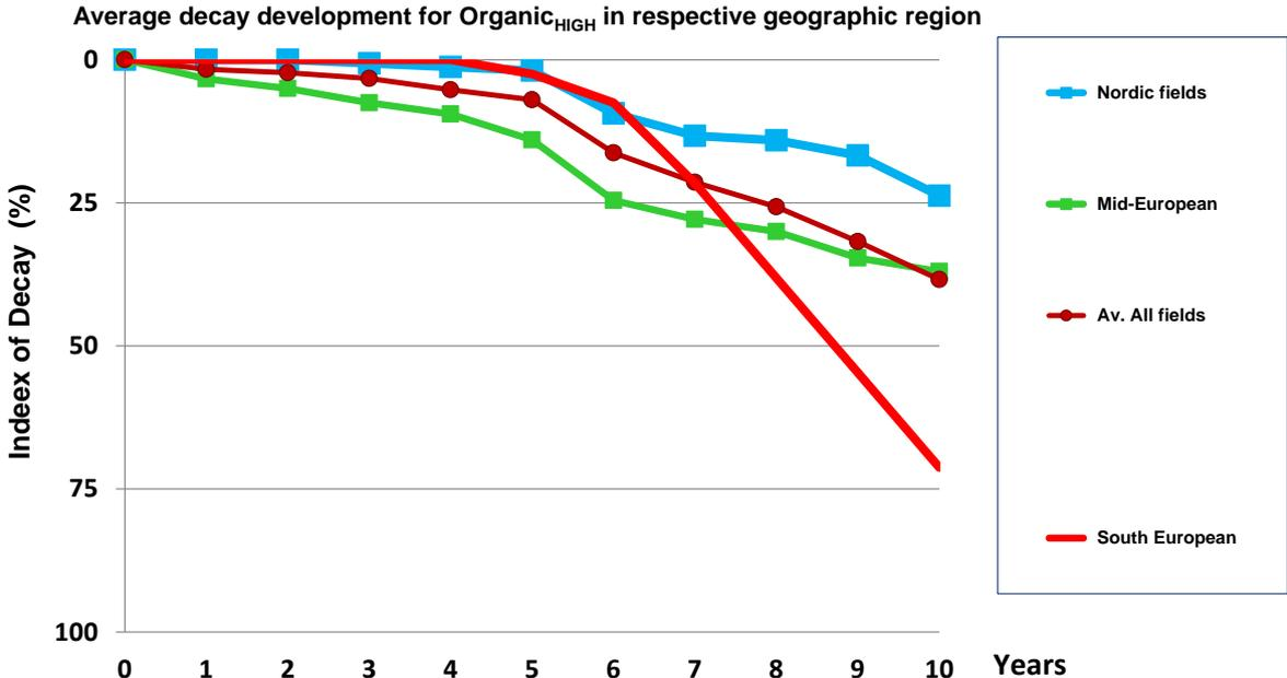
Figure 4: Performance of stakes impregnated with organic preservative to high retention level (levels intended to simulate levels for UC4 that had been obtained from EN 113 tests) in different regions of Europe.
