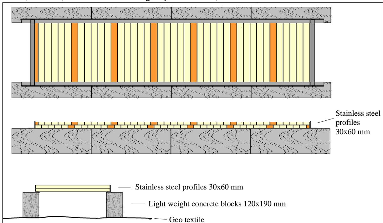
Figure 1: Test rig for double layer test.
