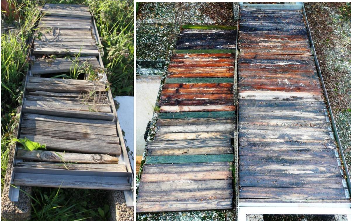
Figure 6: Left: Collapsed test deck in Portugal and Right: Opened up test deck in Hamburg, Germany.
