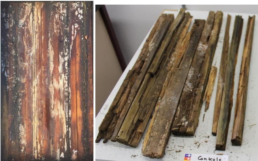
Figure 5: Decay in TMT-UC2 stakes in deck in UK and what remains of Control stakes in Italy after 10 years.
