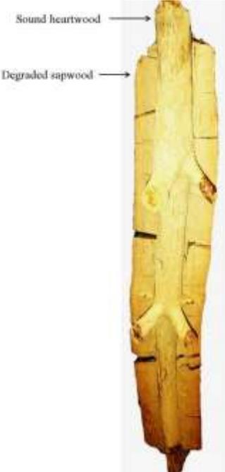
Figure 5. Example of the impact of bacterial decay on a pile (original diameter 130 mm, after 75 years in service and decay, the sound diameter was 35 mm only)
