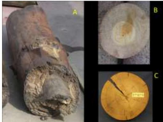
Figure 2. Three pile heads with a soft shell by bacteria decay, for each pile the app. diameter and thickness of the soft shell are given. A: wet broken pine pile head (14 cm / 5 cm); B: wet sawn cross surface pine pile head (18 cm / 6 cm); C: dry cross surface pine pile head (20 cm / 1,5 cm)
