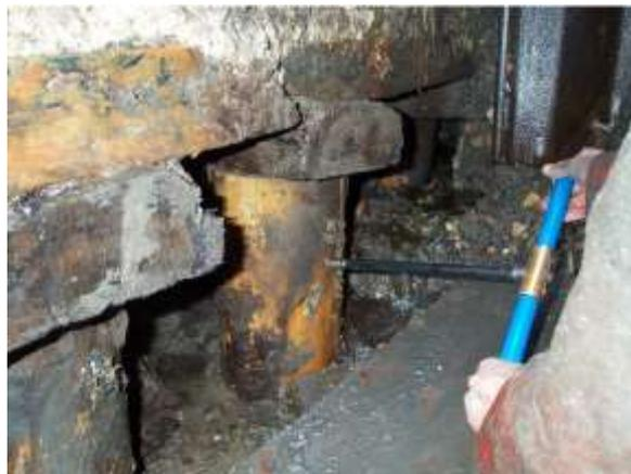
Figure 6. Increment borer (diameter 10 mm)
