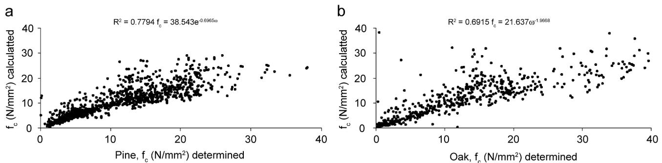
Fig. 8. Model to predict compression strength ( $f_c$ ) from moisture content ( $\omega$ ) in pine (left) and oak (right).
