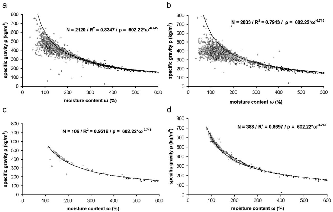
Fig. 5. Relationship between moisture content ( $\omega$ ), specific gravity ( $\rho$ ), and degree of degradation: (a) pine, (b) spruce, (c) alder and (d) oak: (○) sound, (◐) weak, (◑) moderate, (◒) severe, (◓) total disruption of wood structure.
