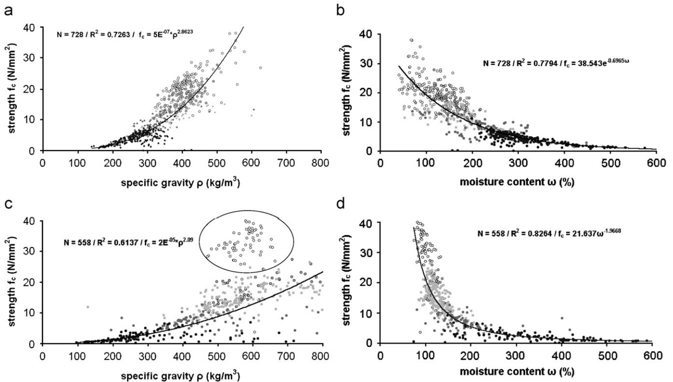
Fig. 6. Relationship between compression strength and specific gravity, moisture content, and degree of degradation: (a and b) pine and (c and d) oak; in (c) fresh material is marked: (○) sound, (◐) weak, (◑) moderate, (◒) severe, (◓) total disrupted wood structure.
