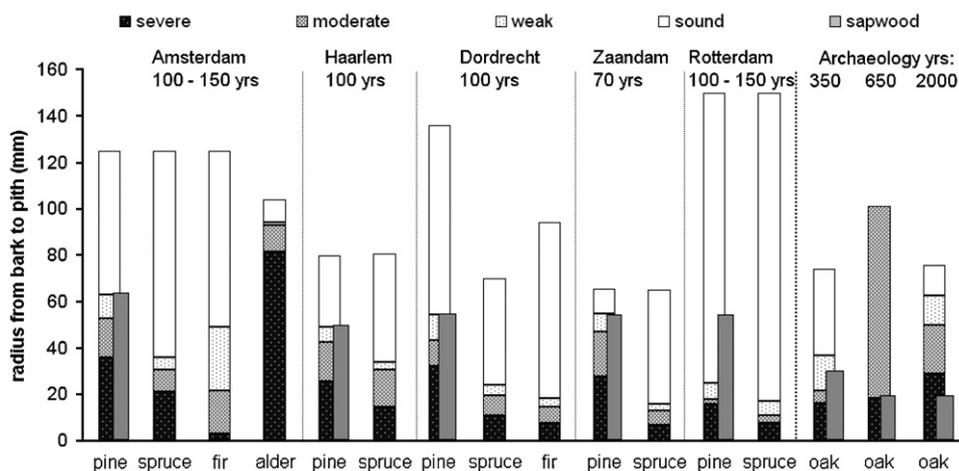
Fig. 4. Mean degree of degradation in pile heads from five Dutch cities (Amsterdam, Rotterdam, 100–150 years; Dordrecht and Haarlem, ca. 100 years; Zaandam, ca. 70 years) and oak from archaeological sites of 350, 650, and 2000 years old. The amount of sapwood is only given for oak and pine. The dimension of the radius is an estimation based on measurements of the pile circumference.
