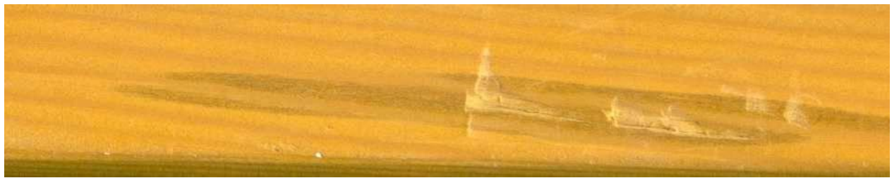
Fig 3 Local increased permeability results in dark spots by semitransparent coatings
