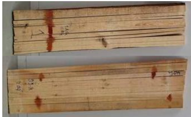
Fig 4: examples of the effect of ponding on stress release in pine boards (75 mm) direct after sawing
